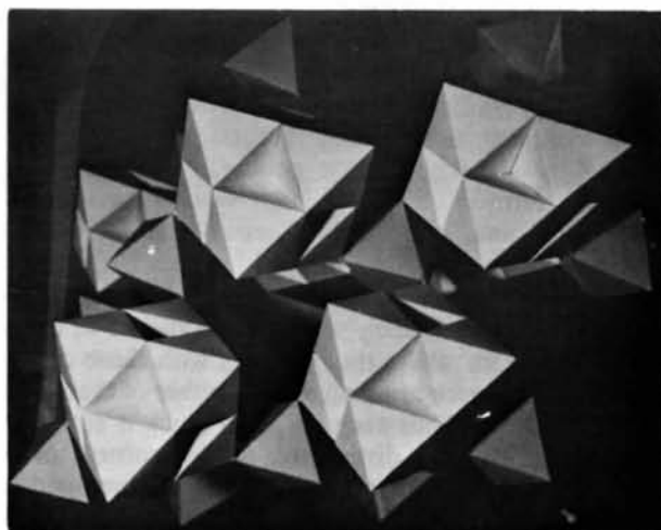
Fig. 2. The arrangement of [\text{W}_6\text{O}_{19}] blocks and [\text{W}_2\text{O}_9] groups, viewed down c .
